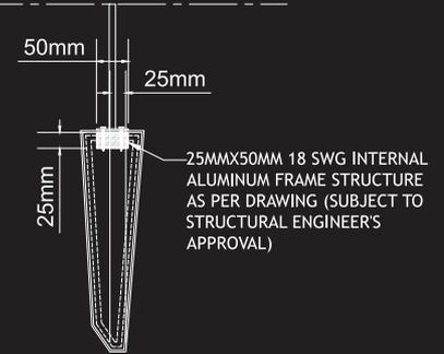
25MMX50MM 18 SWG INTERNAL ALUMINUM FRAME STRUCTURE AS PER DRAWING (SUBJECT TO STRUCTURAL ENGINEER'S APPROVAL)
