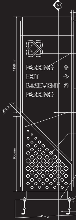
03 FRONT VIEW - DIRECTIONAL PYLON
